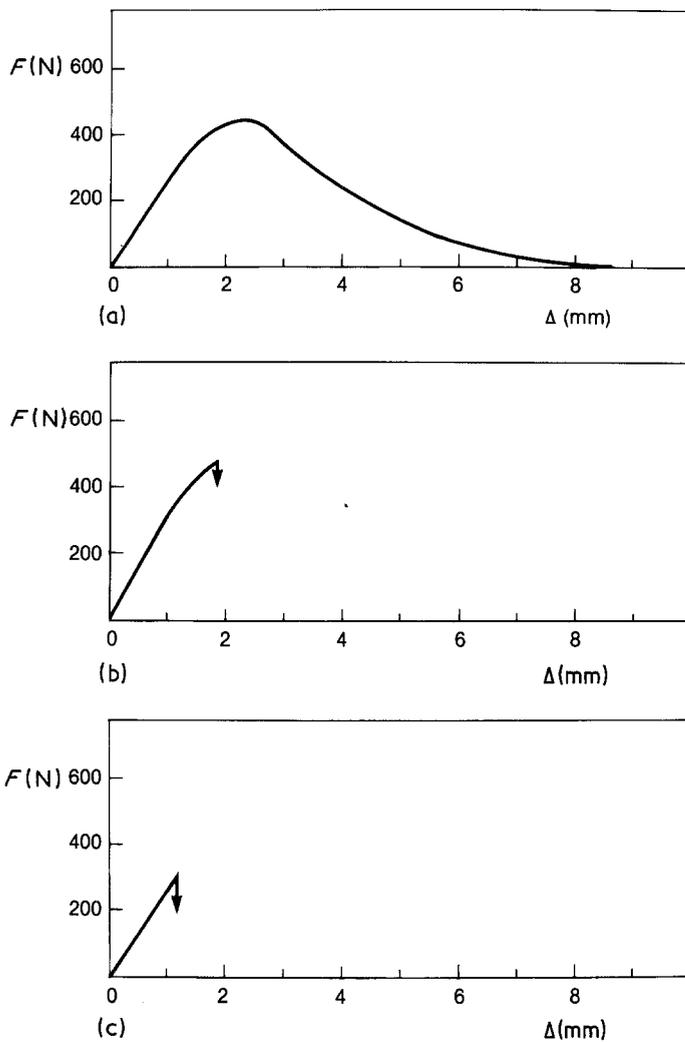
Figure 1 Load-piston displacement curves for PBT/IM 85/15 tested in three-point bending at a piston speed of  $2 \text{ m sec}^{-1}$ . Test temperature: (a)  $25^\circ \text{C}$ ; (b)  $0^\circ \text{C}$ ; (c)  $-30^\circ \text{C}$ .
