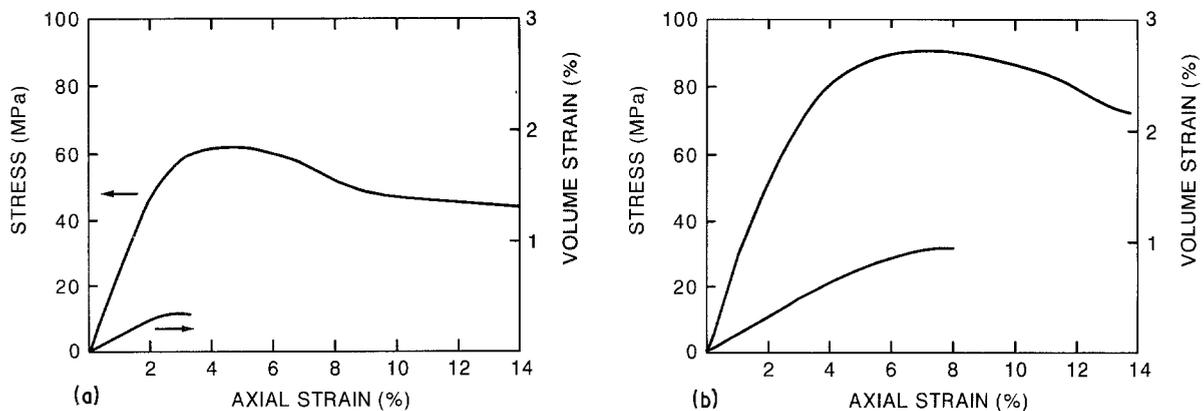
Figure 3 Stress-axial strain-volume strain curves for PBT/PC 45/55 tested at an axial strain rate of  $0.1 \text{ sec}^{-1}$ . Test temperature: (a)  $25^\circ \text{C}$ ; (b)  $-30^\circ \text{C}$ .
