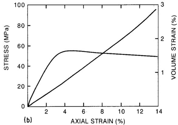
Figure 4 Stress-axial strain-volume strain curves for PBT/IM 85/15 tested at an axial strain rate of  $0.1 \text{ sec}^{-1}$ . Test temperature: (a)  $25^\circ \text{C}$ ; (b)  $0^\circ \text{C}$ ; (c)  $-30^\circ \text{C}$ .
