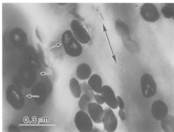
Figure 7 Transmission electron micrograph of PBT/PC/IM 70/15/15 highly deformed at  $-30^{\circ}\text{C}$ . The small arrows indicate cavitated impact modifier particles. The large arrow indicates the tension direction.
