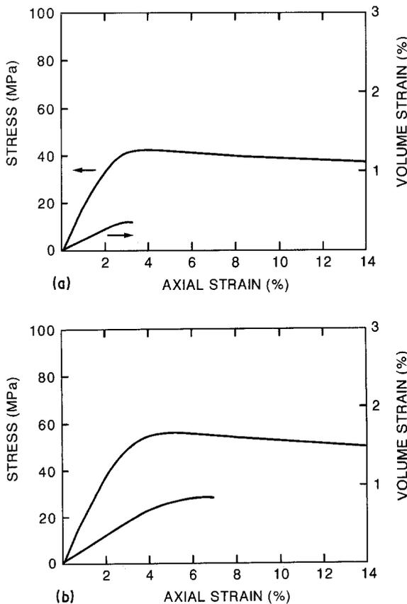
Figure 5 Stress-axial strain-volume strain curves for PBT/PC/IM 70/15/15 tested at an axial strain rate of  $0.1 \text{ sec}^{-1}$ . Test temperature: (a)  $25^\circ \text{C}$ ; (b)  $0^\circ \text{C}$ ; (c)  $-30^\circ \text{C}$ .
