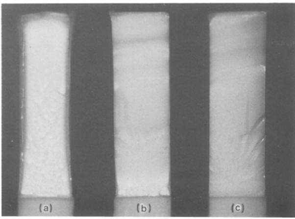
Figure 2 Fracture surfaces of PBT/IM 85/15 tested in three-point bending at a piston speed of  $2 \text{ m sec}^{-1}$ . Test temperature: (a)  $25^\circ \text{C}$ ; (b)  $0^\circ \text{C}$ ; (c)  $-30^\circ \text{C}$ . The notches are visible at the bottom of the photograph.
