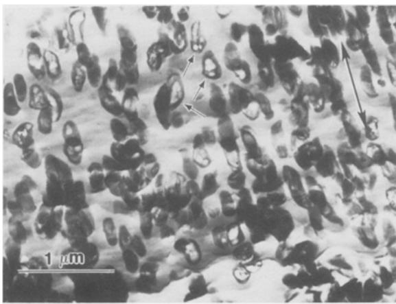
Figure 6 Transmission electron micrograph of PBT/IM 85/15 highly deformed at  $-30^{\circ}\text{C}$ . The small arrows indicate cavitated impact modifier particles. The large arrow indicates the tension direction.
